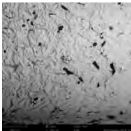
26 | Implant surface (Adin Touareg) with notable light and dark particles (x500).
