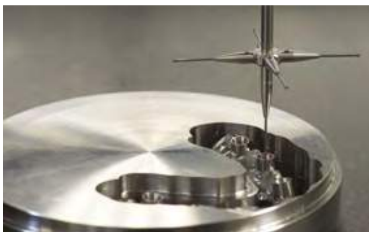
Quality control: three-dimensional measurement of a CAD/CAM bar.
