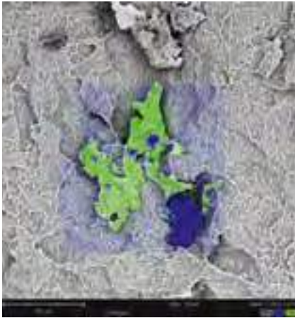
32 | Example of EDX mapping: green = chrome; blue = aluminium (Adin Touareg; x2,500).
